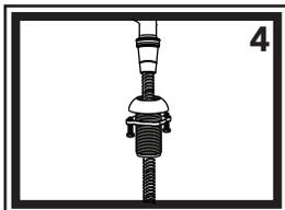
4) Slide hose/sprayer assembly back through the holder from above the deck.
