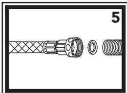
5) Connect to desired 1/2"-Male water source or valve. Make sure the rubber washer is in place in the larger female side of the adapter.
