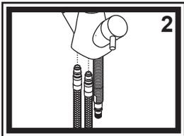
2) Attach the connector hoses to the bottom of the faucet body. Screw the red hose into the left hole (hot inlet) and the blue hose into the right hole (cold inlet), when looking at the faucet body from the front. It is not necessary to use Teflon (plumber's) tape when screwing the hoses into the body, as the o-rings on the tips of the hoses will form a seal.
