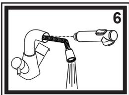
6) Pull the spout head a few inches out from the faucet and unscrew the spout head from the pull-out hose. Aim the hose down into the sink. Turn the water supply back on and allow both hot and cold water to run for at least one full minute without the spout head. While water is running, check all connections for leaks. Replace the spout head. Connections may need re-tightening.
