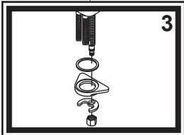
3) Place the faucet in the hole (1 1/4" to 1 3/8" diameter hole - standard size) of the sink, ensuring the rectangular gasket lines up with the base of the faucet body. Slide the round rubber gasket, mounting support, metal horseshoe washer (ensuring that they all line up together) and then the mounting nut onto the mounting shaft, as illustrated and hand tighten the mounting nut. Position the faucet on the sink. Tighten the mounting nut.
