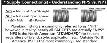
Both NPS and NPT have the same thread angle, shape, and pitch (threads per inch). However, NPS threads are straight (parallel) and NPT threads are tapered (reduced)
