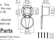
Recessed Cup (Plastic) Lid (Stainless Steel) Hinge Inserts (2x) Mounting Screws (4x)
