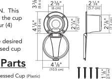
Recessed Cup (Plastic) Lid (Stainless Steel) Hinge Inserts (2x) Mounting Screws (4x)
