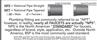
\* Supply Connection(s) - Understanding NPS vs. NPT
