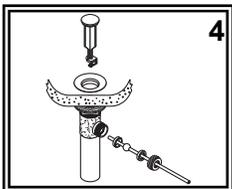
(4) Set the drain plunger in place (see "Drain Plunger" below). Unscrew the pivot ball nut from the pop-up body and remove the spring clip from the pivot ball rod. Leave the white packing ring on and slide the ball nut onto the rod covering the white packing ring. Insert the rod into the hole on the back of the pop-up body. Slide the ball nut in place and tighten securely.
