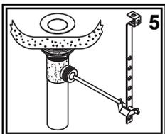
(5) Slide one end of the spring clip onto the end of the pivot rod. Insert the pivot rod into one of the lower holes in the lift rod strap. Secure other end of spring clip onto pivot rod.
