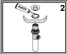
(2) Place a ring of putty around the drain hole in your sink. Insert the threaded end of the drain body up through the drain hole and attach the flange to the body, with the pivot ball nut pointing to the rear of the sink.
