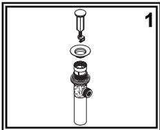
(1) Unscrew flange from drain body. Leave large black washer, white friction ring and locknut on drain body.
