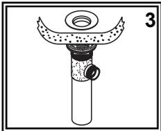
(3) Tighten the locknut from under the sink until the black rubber washer seats securely inside the sink drain hole. Wipe away excess putty. Tighten brass locknut with a wrench.
