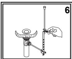
(6) Slide lift rod down through the hole in faucet. Insert bottom of lift rod into hole on the top of the lift rod strap (see "Adjusting The Lift Rod" below). Tighten with thumb screw.
