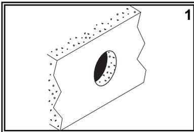
(1) Hold spigot on the wall where desired. Make sure to leave enough room for your hose to hang freely. Drill 1" hole in the wall in the desired location.
