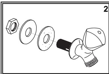
(2) Make sure male nipple is tight into the spigot. Slip nipple through the hole in the wall. Make sure gasket properly lines up with the back of the spigot. From the back side of the wall, slide the rubber and metal washers onto the nipple. Thread the lock nut onto the brass nipple and tighten.
