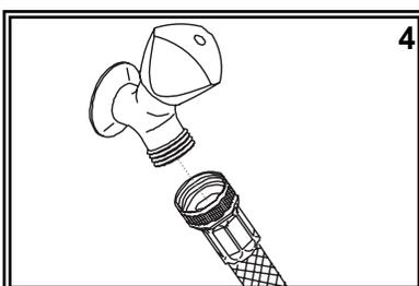
(4) Attach your garden hose to the bib. Turn the water supply on. While water is running, check all connections for leaks. Connections may need re-tightening.
