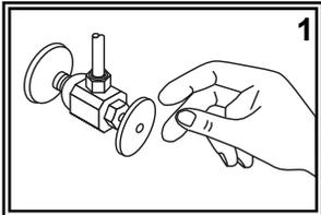
(1) Turn off the water supply to your existing faucet (this procedure will vary depending on the specific plumbing system installed on your boat). Cover the sink drain to prevent any small parts or debris from falling in. Remove your existing faucet, taking care not to damage your existing water lines. Clean sink area in preparation for new faucet.
