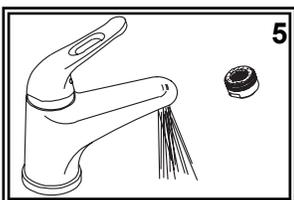
(5) After installation is complete, remove the aerator. Be careful not to scratch the finish. Turn the water supply back on and allow both hot and cold water to run for at least one full minute. While water is running, check all connections for leaks. Replace aerator. Connections may need re-tightening.
