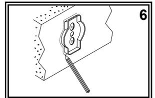
(1) Hold item on the wall where desired. With a pencil, lightly trace a circle completely around the base of the item. Remove the item. Hold a mounting bracket directly in the center of the outline (see figure 6). Trace a circle around the mounting bracket and the two mounting screw holes.
