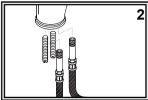
(2) Screw the mounting bolt into the bottom of the faucet. One end of the bolt is slotted to allow the use of a screwdriver to secure. Screw both connector hoses into the bottom of faucet (note: it is NOT necessary to use Teflon (Plumber's) tape on this connection as the o-rings will prevent leaks). Use a wrench or pliers on the hex nut molded into the brass shaft portion of the hoses. Do NOT attempt to tighten by turning the hose itself.
