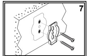
(2) Mount the bracket as shown (see figure 7). For mounting into wood, fiberglass, or other solid surface, drill a 1/8" starter hole and attach the bracket to the wall.
