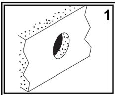
(1) Hold elbow on the wall where desired. Make sure to leave enough room for the hose to hang freely and extend into the shower. Drill 1" hole in the bulkhead in the desired location.
