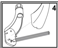
(4) Remove the bracket cover on the post. Hold the bottom post on the wall where desired. Note, "top" and "bottom" posts are identical. Either post can be used as "top" or "bottom". With a pencil, lightly trace a circle around the two screw holes in the post. Remove the post.
