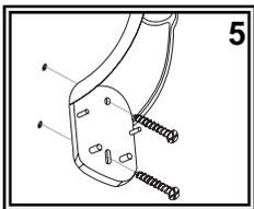
(5) Mount the post as shown. For mounting into fiberglass or other solid surface, drill a 1/8" starter hole and attach the bracket to the wall.
