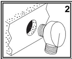
(2) Slip nipple on the back of the elbow through the hole in the bulkhead.
