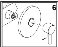
(6) Replace handle and wall plate onto valve assembly. Slide wall plate back onto the trim sleeve. Be careful not to damage the wall plate gasket. Tighten the handle screw and replace the blue/red cap. It may be necessary to secure the valve inside the wall to prevent movement. This procedure will vary depending on the specific design of your boat. Suggestions: Use the screw-holes molded into the valve. Use strapping material. Wedge item in place.
