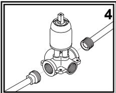
(4) Connect hot/cold water supply lines (not provided) to the inlet tubes. The inlet tubes are the 1/2" NPT-Female tubes on the left and right sides of the valve. Wrap the fittings with Teflon (Plumber's) tape. This procedure will vary depending on the specific plumbing system installed on your boat.
