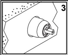
(3) From the back side of the bulkhead, slide the valve assembly through the hole in the bulkhead. Note that the brass valve is stamped with "UP". Make sure that the "UP" is on the top side when positioned.
