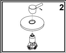
(2) Remove handle and wall plate from valve assembly. Remove the blue/red cap and loosen the set screw behind it. Slide handle off the cartridge. Slide wall plate off the trim sleeve. Be careful not to damage the wall plate gasket.
