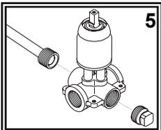
(5) Connect 1/2" NPT water line from the shower head or bulkhead elbow (not included) to the shower head (top) port. Wrap the fitting on the water line with Teflon (Plumber's) tape. Thread tub port plug into the tub port (bottom) (if you are not using a tub spout with this installation). Wrap the plug with Teflon (Plumber's) tape.
