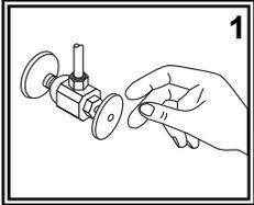
(1) Turn off the water supply to your existing faucet (this procedure will vary depending on the specific plumbing system installed on your boat). Remove old shower set.
