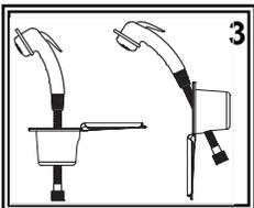
**Deck Mount**—Place into the hole with the hinge pointing in the desired direction for the lid to easily lay open when in use. *Please note:* The trigger will stick out through the side hole when the sprayer is resting in the recessed cup. It is important to ensure there is ample clearance for the trigger, in order to prevent accidental discharge. Secure recessed cup and lid using the provided four (4) screws.
