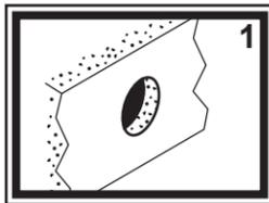
1) Check desired position to ensure adequate space under the deck or inside the wall for the recessed cup plus the item being installed inside the cup. Drill 2 7/8" to 3" hole in the desired location.
