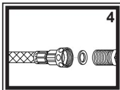
3) Slide hose/sprayer assembly through the appropriate hole in the recessed cup, as illustrated.
