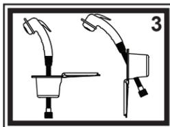
**Deck Mount**— Place into the hole with the hinge pointing in the desired direction for the lid to easily lay open when in use. **Please note:** The trigger will stick out through the side hole when the sprayer is resting in the recessed cup. It is important to ensure there is ample clearance for the trigger, in order to prevent accidental discharge. Secure recessed cup and lid using the provided four (4) screws.
