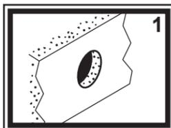
1) Check desired position to make sure there is enough room for the hose to gather under the deck or inside the wall without getting caught on anything. Drill 2 7/8" to 3" hole in the desired location.
