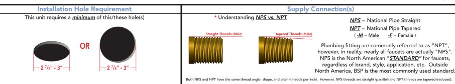
Straight Pipe thread is commonly found on faucets, showerheads, hose connections and fittings. Tapered Pipe thread is commonly found on pipe ends, nipples and fittings (i.e. couplings, elbows, tees, etc.). Straight Pipe threads need a gasket or o-ring to create a seal. Both styles require sealant or plumber's tape for optimal seal. While NPS and NPT threads will engage, they do not seal properly with each other.
