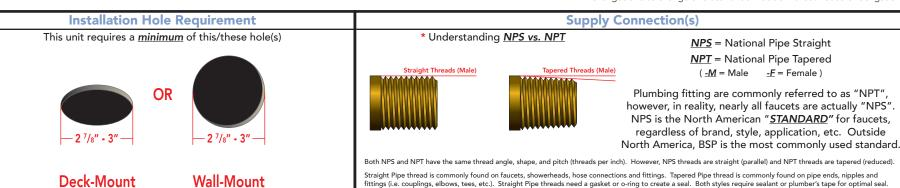
Straight Pipe thread is commonly found on faucets, showerheads, hose connections and fittings. Tapered Pipe thread is commonly found on pipe ends, nipples and fittings (i.e. couplings, elbows, tees, etc.). Straight Pipe threads need a gasket or o-ring to create a seal. Both styles require sealant or plumber's tape for optimal seal. While NPS and NPT threads will engage, they do not seal properly with each other.
