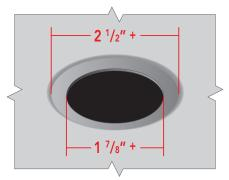
The Drain Size is a standardized term used to refer to the category of drain body sizes. The actual hole in the sink is typically <sup>1</sup>/<sub>16</sub>" to <sup>1</sup>/<sub>2</sub>" larger diameter than the "Drain Size".
