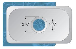
The Drain Size is a standardized term used to refer to the category of drain body sizes. The actual hole in the sink is typically <sup>1</sup>/<sub>16</sub>" to <sup>1</sup>/<sub>2</sub>" larger diameter than the "Drain Size".
