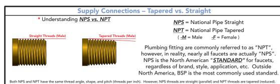
Straight Pipe thread is commonly found on faucets, showerheads, hose connections and fittings. Tapered Pipe thread is commonly found on pipe ends, nipples and fittings (i.e. couplings, elbows, tees, etc.). Straight Pipe threads need a gasket or o-ring to create a seal. Both styles require sealant or plumber's tape for optimal seal. While NPS and NPT threads will engage, they do not seal properly with each other.
