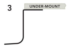
This Flange Style allows for "Under-Mounting" of the sink to the counter-top
