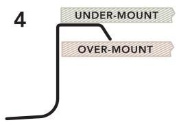
This Flange Style allows for either "Over-Mounting" or "Under-Mounting" of the sink on the counter-top
