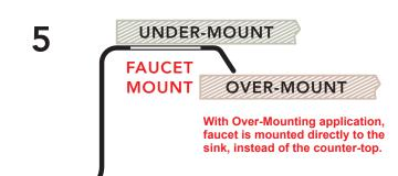
This Flange Style allows for either "Over-Mounting" or "Under-Mounting" of the sink on the counter-top
