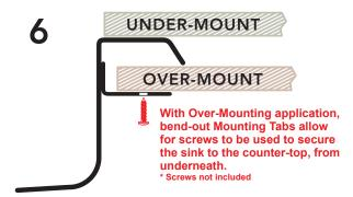
This Flange Style allows for either "Over-Mounting" or "Under-Mounting" of the sink on the counter-top
