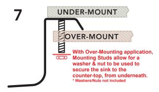
This Flange Style allows for either "Over-Mounting" or "Under-Mounting" of the sink on the counter-top
