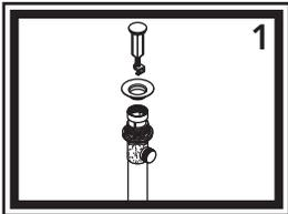
1) Unscrew flange from drain body. Leave large black gasket, white friction ring and lock nut on drain body.
