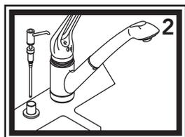
2) To fill the soap dispenser, lift the pump nozzle and plastic pump out through the top side. Pour in liquid soap (or hand lotion). Replace pump and pump nozzle. NOTE: If soap (or hand lotion) is too thick, pump may not function properly, dilute with water.
