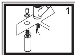
1) Insert the bottle, with the brass shaft, lock nut, and washer, up from below. From the top, set the escutcheon onto the brass shaft. Tighten the housing down onto the shaft. Tighten the lock nut under the sink.
