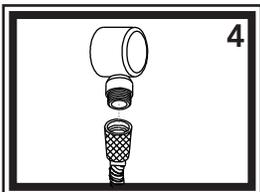
4) Attach your 1/2" hose to the connector. Turn the water supply on. While water is running, check all connections for leaks. Connections may need re-tightening.
