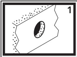
1) Hold elbow on the wall where desired. Make sure to leave enough room for your hose to hang freely and extend into the shower. Drill 1" hole in the bulkhead in the desired location.
