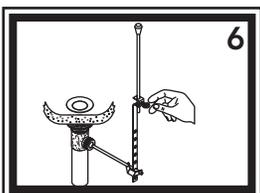
6) Slide lift-rod down through the hole in faucet. Insert bottom of lift-rod into hole on the top of the lift-rod strap (see "Adjusting The Lift-Rod" below). Tighten with thumb screw.
