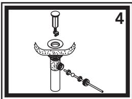
4) Set the drain plunger in place (see "Drain Plunger" below). Unscrew the pivot ball nut from the pop-up body and remove the spring clip from the pivot ball rod. Leave the white packing ring on and slide the ball nut onto the rod covering the white packing ring. Insert the rod into the hole on the back of the pop-up body. Slide the ball nut in place and tighten securely.
