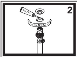
2) Place a ring of putty around the drain hole in your sink. Insert the threaded end of the drain body up through the drain hole and attach the flange to the body, with the pivot ball nut pointing to the rear of the sink.
