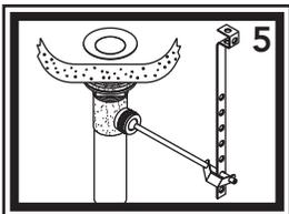
5) Slide one end of the spring clip onto the end of the pivot rod. Insert the pivot rod into one of the lower holes in the lift rod strap. Secure other end of spring clip onto pivot rod.
