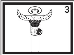
3) Tighten the lock nut from under the sink until the black rubber gasket seats securely inside the sink drain hole. Wipe away excess putty. Tighten brass lock nut with a wrench.
