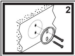
2) Mount the bracket as shown (see figure 2). For mounting into wood, fiberglass, or other solid surface, drill a 1/8" starter hole and attach the bracket to the wall.
