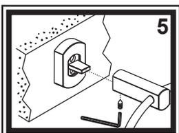
3) Slide the bodies back onto the bases with the set screws pointing down (see figure 5). If both bodies do not properly align with the bases, one or both bases may need to be slightly adjusted. Slightly loosen the mounting screws securing one of the bases to the wall, allowing the base to shift positioning within the mounting screws, correct the base's location on the wall and re-tighten the mounting screws. Tighten the set screws to secure the bodies to the bases.
