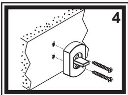
2) Secure the bases to the wall. For mounting into wood, fiberglass, or other solid surface, drill a 1/8" starter hole and attach the bases to the wall as shown with the provided screws (see figure 4).
