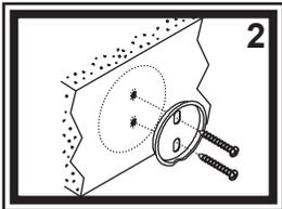
2) Secure the bracket to the wall. Note that the bracket has a dimpled edge, which is the bottom. For mounting into wood, fiberglass, or other solid surface, drill a 1/8" starter hole and attach the bracket to the wall as shown (see figure 2). Carefully erase the pencil circle from tracing around the base.
