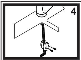
4) Attach weight to hose approximately 1 1/2" to 2" up from the bottom of the arch. Adjust position as desired. Weight should be installed to prevent hose kinking and for easy hose return.
