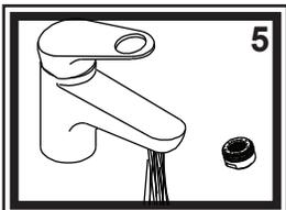
5) After installation is complete, remove the aerator. Be careful not to scratch the finish. Turn the water supply back on and allow both hot and cold water to run for at least one full minute. While water is running, check all connections for leaks. Replace aerator. Connections may need re-tightening.
