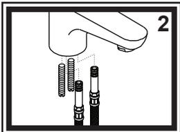
2) Screw mounting bolts into the bottom of the faucet. One end of the bolt is slotted to allow the use of a screwdriver to secure. Screw both connector hoses into the bottom of faucet (note: it is NOT necessary to use Teflon (Plumber's) tape on this connection as the o-rings will prevent leaks). Use a wrench or pliers on the hex nut molded into the brass shaft portion of the hoses. Do NOT attempt to tighten by turning the hose itself.
