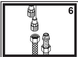
7) Unscrew the spout head from the flex hose. Turn the water supply back on and allow both hot and cold water to run for at least one full minute without the spout head. While water is running, check all connections for leaks. Replace the spout head. Connections may need re-tightening.
