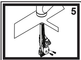
5) Attach metal weight to hose. Adjust position as desired. Weight must be installed to prevent hose kinking and for easy hose return.
