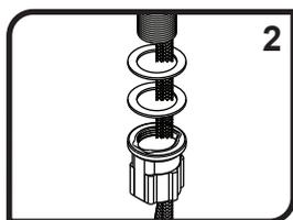
2) From under the sink, slide the rubber and metal Washers up the Mounting Shaft. Thread the Mounting Nut onto the Mounting Shaft and loosely tighten. Confirm the proper position of the faucet from above the sink. Tighten the easy grip Mounting Nut by hand or with an adjustable wrench or pliers. It may be necessary to re-adjust the faucet position by slightly loosening the Mounting Nut, adjusting to the desired location, then re-tightening the Mounting Nut.
