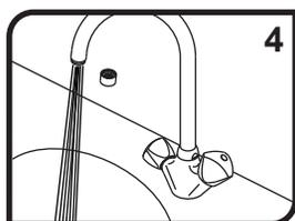
4) After installation is complete, unscrew the aerator. Be careful not to scratch the finish. Turn the water supply back on and allow both hot and cold water to run for at least one full minute. While water is running, check connections for leaks. Replace aerator. Connections may need re-tightening. Turn handle on/off, rotate spout side-to-side a few times to verify proper function.
