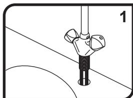
1) Remove the Mounting Nut (Easy Grip), metal and rubber Washers from the Mounting Shaft, if already attached. Place the faucet through the hole in your sink/counter-top, making sure the O-Ring remains recessed in the base of the Body. Position so that the O-Ring in the base forms a seal all the way around the hole.
