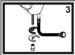
3) Place your new faucet through the hole in your sink. Make sure the black gasket properly lines up with the bottom of the faucet. From under the sink, slide the rubber horseshoe washer then the metal horseshoe washer onto the mounting bolt. Adjust faucet position on the sink as desired. Thread the lock nut onto the mounting bolt and tighten. It may be necessary to re-adjust the faucet position by slightly loosening the lock nut, adjusting to desired location, then re-tightening the lock nut.
