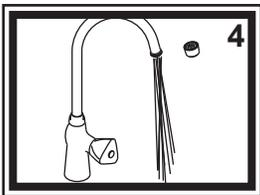
4) After installation is complete, remove the aerator. Be careful not to scratch the finish. Turn the water supply back on and allow the water to run for at least one full minute. While water is running, check all connections for leaks. Connections may need re-tightening.
