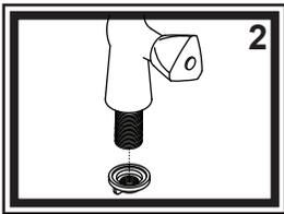
2) Place the faucet in the hole (1 3/8" diameter hole - standard size) of the sink. From under the sink, thread the lock nut onto the inlet tube and tighten. It may be necessary to re-adjust the faucet position by slightly loosening the lock nut, adjusting to desired location, then re-tightening the lock nut.
