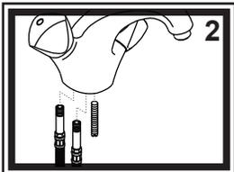
2) Screw mounting bolt into the bottom of the faucet. One end of the bolt is slotted to allow the use of a screwdriver to secure. Screw both connector hoses into the bottom of faucet (note: it is NOT necessary to use Teflon (Plumber's) tape on this connection as the o-rings will prevent leaks). Use a wrench or pliers on the hex nut molded into the brass shaft portion of the hoses. Do NOT attempt to tighten by turning the hose itself.
