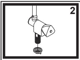
2) Place the faucet in the hole (1" diameter hole) in your sink. From under the sink, thread the lock nut onto the inlet tube and tighten. It may be necessary to re-adjust the faucet position by slightly loosening the lock nut, adjusting to desired location, then re-tightening the lock nut.
