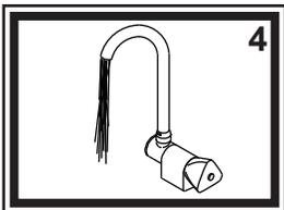
4) Turn the water supply back on and allow the water to run for at least one full minute. While water is running, check connections for leaks. Connections may need re-tightening.
