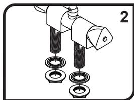
2) From under the sink, slide the rubber Washers and thread the Mounting Nuts onto the Inlet Tubes and hand-tighten. Confirm the proper position of the faucet from above the sink. Tighten the Mounting Nuts with an adjustable wrench or pliers. It may be necessary to re-adjust the faucet position by slightly loosening the Mounting Nuts, adjusting to the desired location, then re-tightening the Mounting Nuts.
