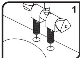
1) Place the faucet through the hole in your sink/counter-top. If the Mounting Nuts and rubber Washers are already on the Inlet Tubes, remove them before placing unit in the wholes.
