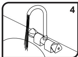
4) Turn the water supply on and allow both the hot and cold water to run for at least one full minute. While water is running, check connections for leaks. Connections may need re-tightening. Turn handles on/off, rotate spout side-to-side and up-and-down a few times to verify proper function.
