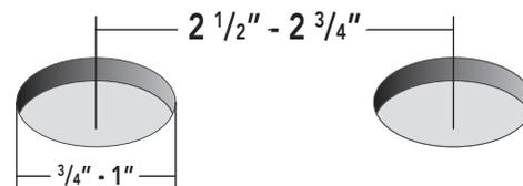
Your existing sink/counter-top may have additional hole(s) per-drilled, which may not be required for this installation. If so, you may be able to utilize a deck/cover plate or an additional accessory (i.e. soap dispenser) to utilize the extra hole(s). We offer a variety of deck/cover plates and soap dispensers to coordinate with your faucet and decor.
