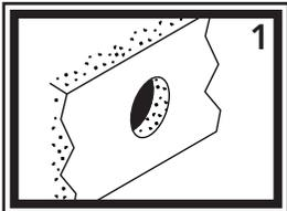
1) Hold spigot on the wall where desired. Make sure to leave enough room for your hose to hang freely. Drill 1" hole in the wall in the desired location.
