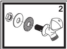
2) Make sure male nipple is tight into the spigot. Slip nipple through the hole in the wall. Make sure gasket properly lines up with the back of the spigot. From the back side of the wall, slide the rubber and metal washers onto the nipple. Thread the lock nut onto the nipple and tighten.
