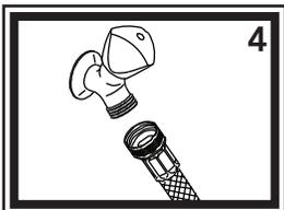
4) Attach your garden hose to the bib. Turn the water supply on. While water is running, check all connections for leaks. Connections may need re-tightening.
