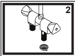
2) Place your new faucet through the holes in your sink. From under the sink, thread the lock nuts onto the brass inlet tubes and tighten. It may be necessary to re-adjust the faucet position by slightly loosening the lock nuts, adjusting to desired location, then re-tightening the lock nuts.
