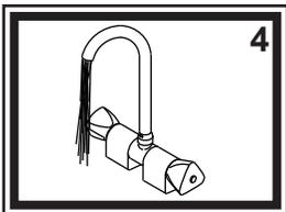
4) Turn the water supply back on and allow both hot and cold water to run for at least one full minute. While water is running, check all connections for leaks. Connections may need re-tightening.
