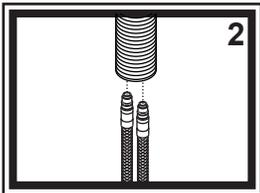
2) If necessary, screw the connector hoses to the bottom of the faucet body. Screw the red hose into the left hole (hot inlet) and the blue hose into the right hole (cold inlet), when looking at the faucet from the front. It is not necessary to use Teflon (plumber's) tape when screwing the hoses into the body, as the o-rings on the tips of the hoses will form a seal.
