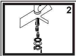
2) Place the faucet in the center hole (1 3/8" diameter hole - standard size) of the sink. Pull the flex hose all the way up until the hose stops. Slide the black rubber washer and then the metal washer onto the mounting shaft. Screw the brass lock nut onto the mounting shaft with the two screws pointing up, as illustrated. Hand tighten the brass lock nut. Position the faucet on the sink and tighten the lock nut screws with a screwdriver. **CAUTION: DO NOT OVER TIGHTEN THE SCREWS.**
