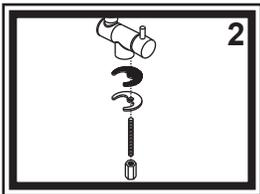
2) Place the faucet in the hole (1" diameter hole) in your sink. From under the sink, slide the rubber horseshoe and meal horseshoe washers up the mounting rod with the washers wrapping around the inlet hoses. Thread the mounting nut onto the mounting rod and tighten. It may be necessary to re-adjust the faucet position by slightly loosening the mounting nut, adjusting to desired location, then re-tightening the mounting nut.
