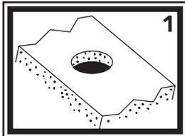
1) Check desired position to make sure there is enough room for the hose to gather under the deck without getting caught on anything. Drill 1" hole in the deck in the desired location.
