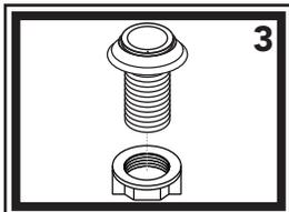
3) Slip hose nest through the hole in the deck. Make sure hose nest collar properly lines up with the hose nest shaft. From under the deck, thread the lock nut onto the hose nest shaft and tighten.
