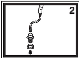
2) Remove hose nest assembly from hose/sprayer assembly. Unscrew 1/2" adapter from hose and pull hose out through the top side of the hose nest shaft. Remove lock nut from hose nest shaft.
